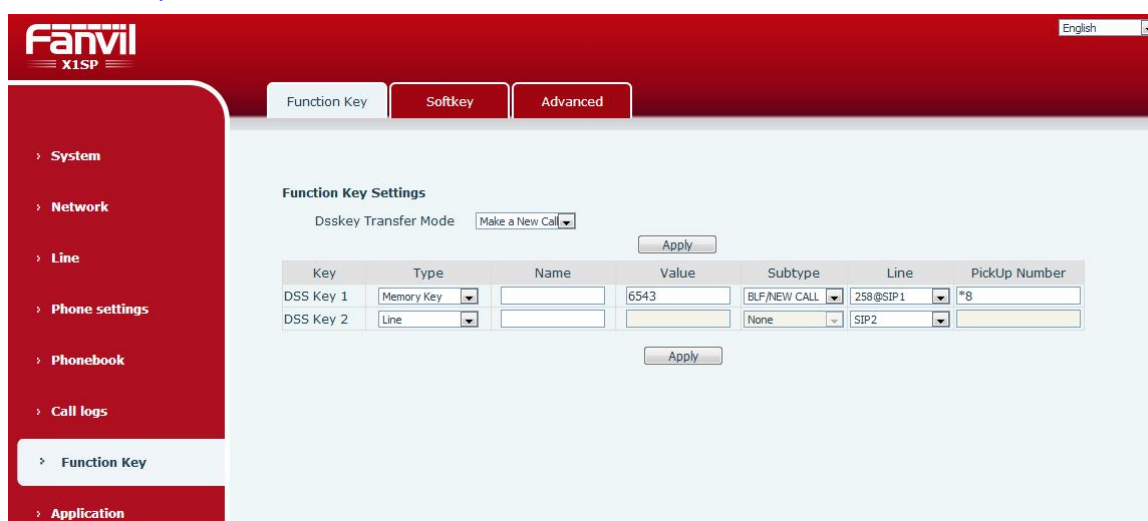
Picture 61 - Web page configuration BLF function key
